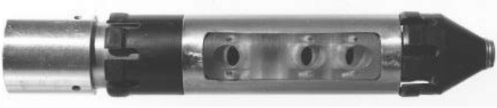
Figure 7.14 Example of probe design for a stud inspection from the bore side. Reprinted by permission of Westinghouse Electric Company LLC.
