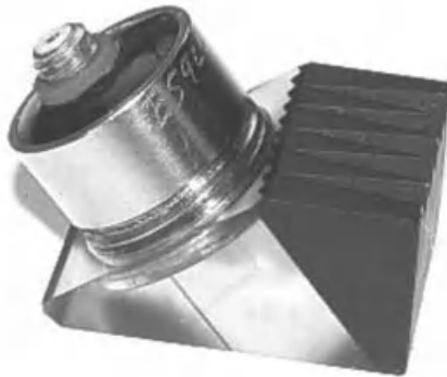
Figure 2.1 A typical angle beam probe: a transducer attached to a wedge.
