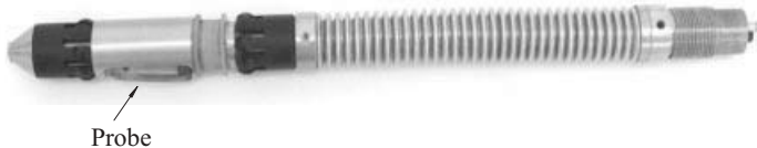
Figure 8.12 Example of a probe assembly for SGT inspection. Reprinted by permission of Westinghouse Electric Company LLC.
